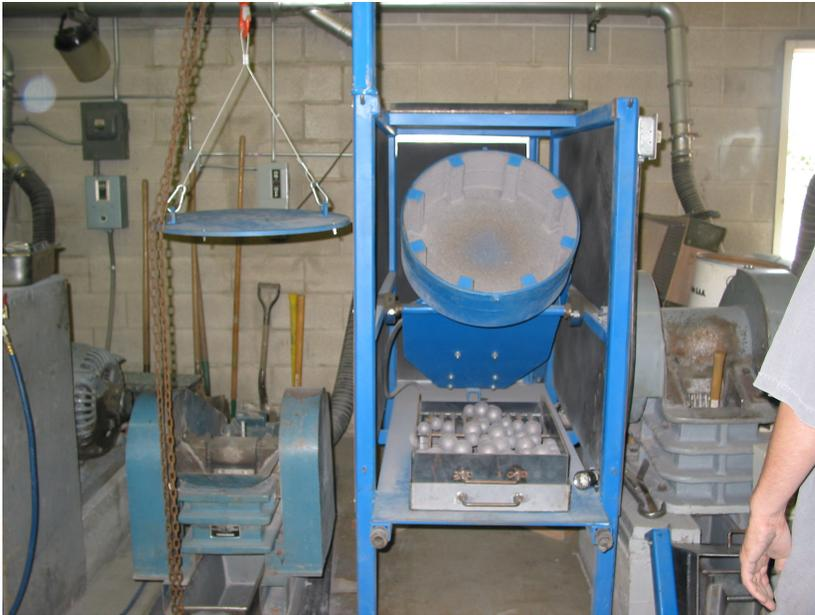
**Figure 2 – SAGDesign Test Mill**
