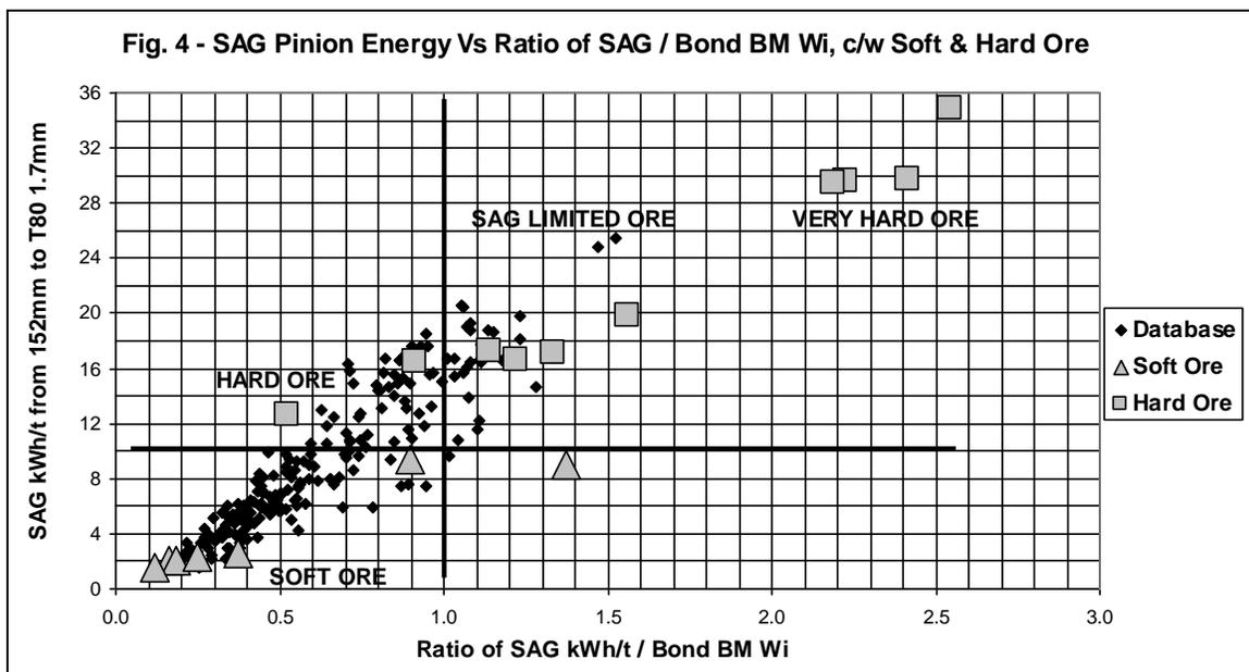
To emphasize this point, Figure 4 has been prepared. Here the SAGDesign database is presented differently with SAG kWh/t being plotted against the ratio of SAG kWh/t to Bond Ball Mill Wi. Looking at the data this way shows the extreme differences between ores at the same ball mill hardness.
