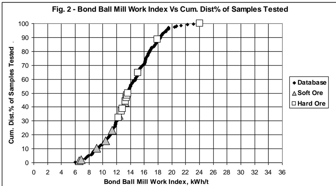
Here both the hard ore and the soft ore (in the SAG mill) overlapped other hardness ranges for the Bond BM Wi database. Because the shape of these curves are so different it proves that the data generated for each sample can only be used in the context of both measurements together. When the Bond Rod Mill Work Index is used instead of the SAGDesign measurement, the Rod Mill Wi variability graph will look more like Figure 2 (McKen et al., 2006) than
