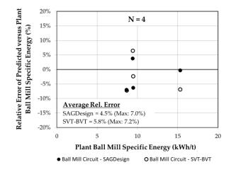
Figure 3 Accuracy of the SVT-BVT compared to the SAGDesign Test Results from Plant Benchmarking
